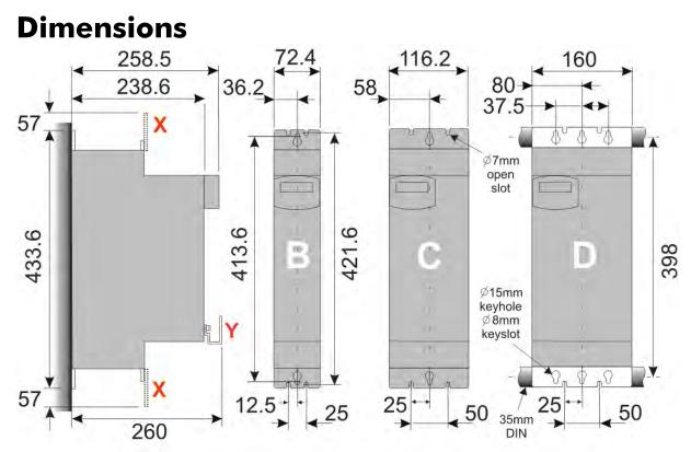
Dimensions are in millimeters (X: Power Bracket - 890 Installation Kit, Y: Control Bracket)
